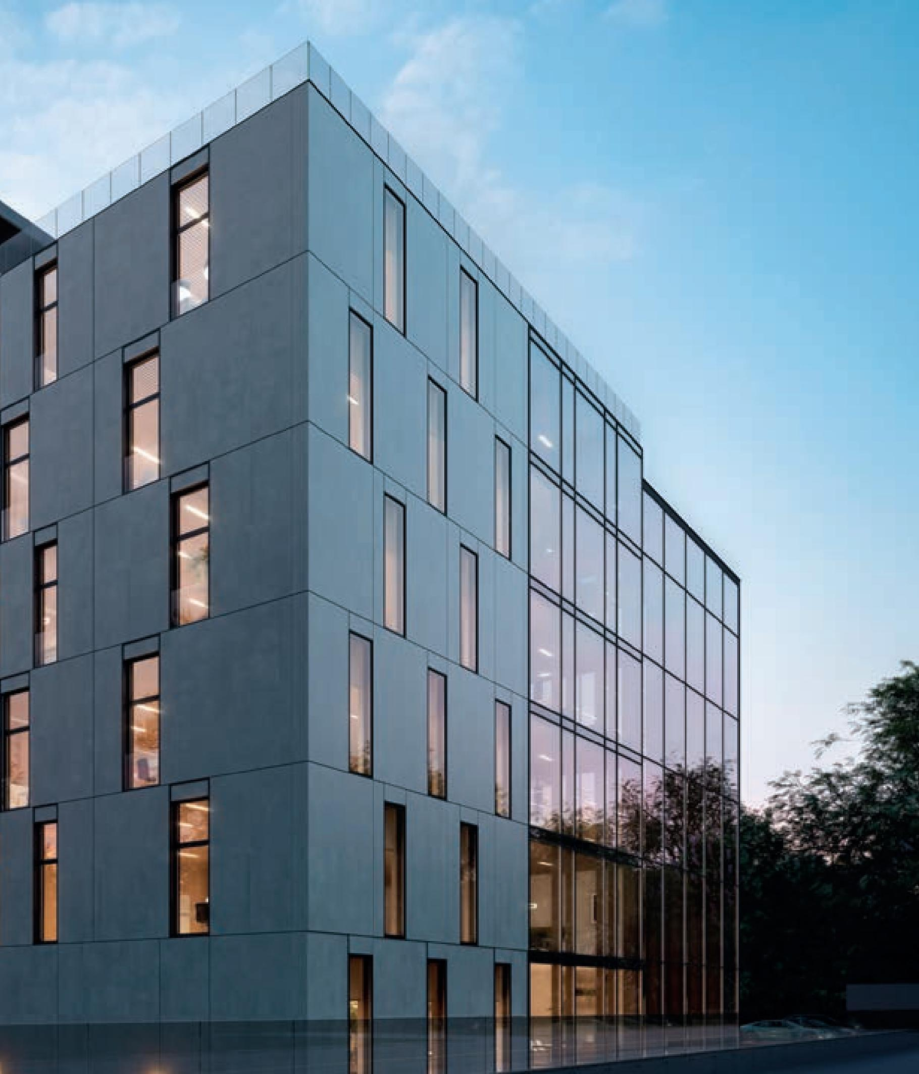
VISTA ESTERNA FACCIATE SCHÜCO FWS 35 PD.HI - UDC 80.SI<sub>xps</sub> - FWS 60.SI - AOC 60 ST - PARAPETTO SCHÜCO AR FG 300
